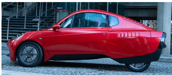
Figure 13: The Riversimple Rasa, small hydrogen fuel cell car with a 300 mile range
